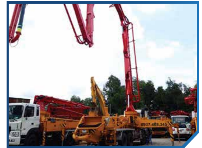
Equipment: Concrete Pump Origin: Vietnam; Quantity: 04 Capacity: 60 - 90m 3 /h Function: Pumping concrete
