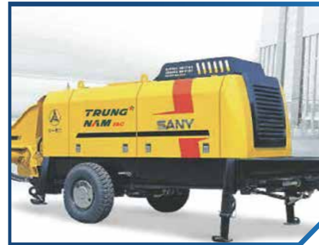
Equipment: Static pump Origin: Vietnam; Quantity: 04 Capacity: 60 - 90m 3 /h Function: Pumping concrete
