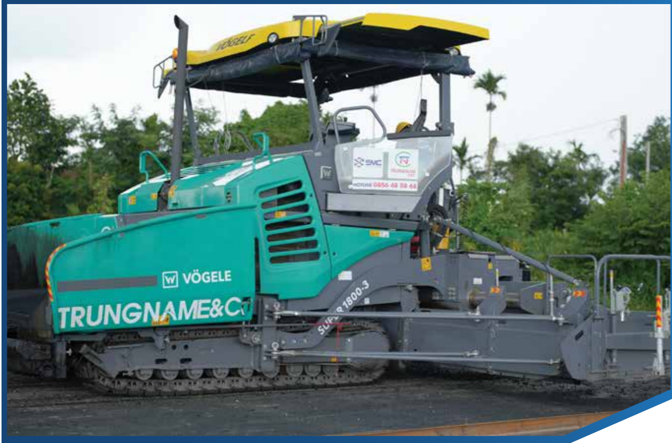
Equipment: Concrete Paver (asphalt VÖGELE model Super 1800-3) Origin: Germany Quantity: 01
