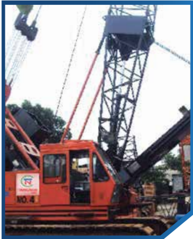
Equipment: CKN(R6G) Rotary Drilling Rig Origin: Japan Quantity: 04
