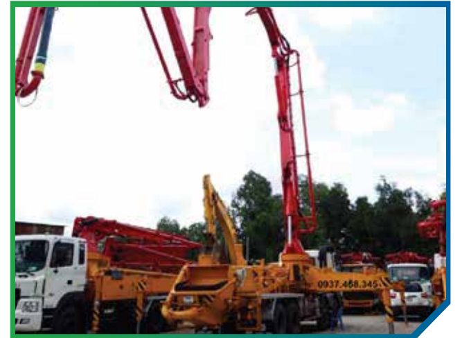
Equipment: Concrete Pump Origin: South Korea - Quantity: 06 Capacity: 60 - 90 - 170m 3 /h Function: Pumping concrete
