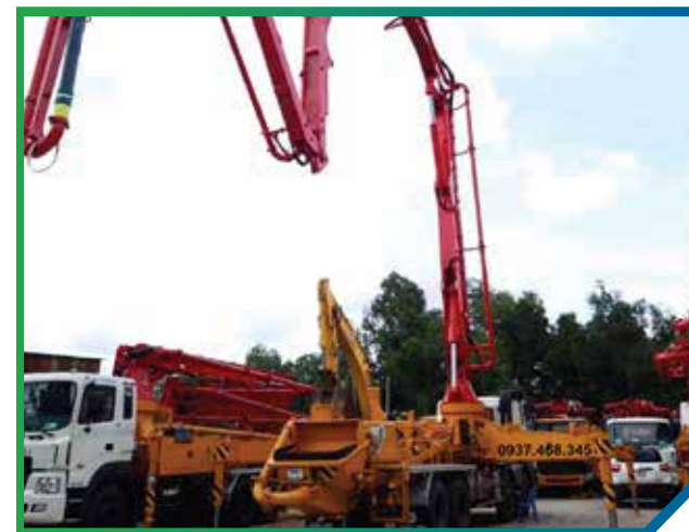
Equipment: Concrete Pump Origin: Vietnam; Quantity: 04 Capacity: 60 - 90m3/h Function: Pumping concrete
