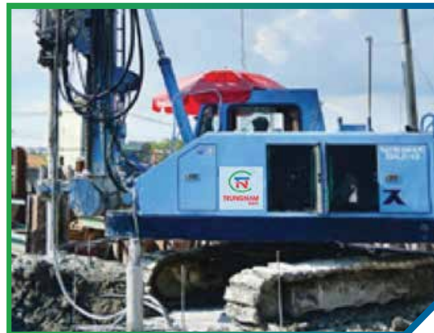
Equipment: XMD Piling Rig Origin: Japan - China - Quantity: 04 Function: Drilling, excavating, and cutting rock for foundations
